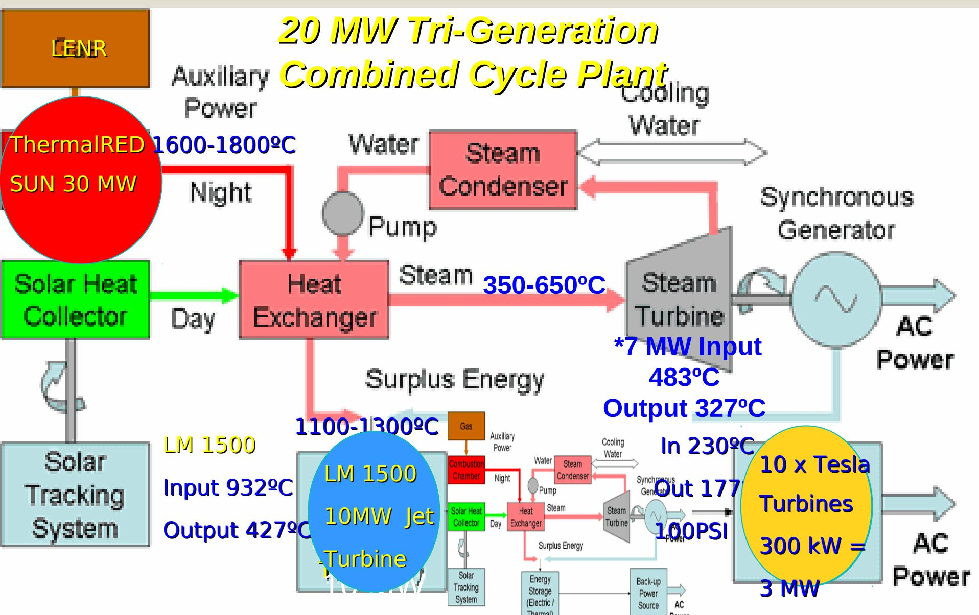
\*7 MW Steam: pressure of 250 PSI an inlet pressure of 850 PSIG @ 483 DEG C, and induction pressure of 650 PSIG @ 327 DEG C, with a Flow of 130,000/90,000 LBS/HR
