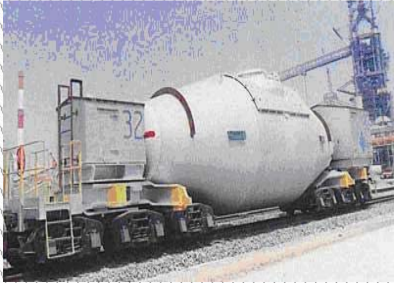
Torpedo Rail Car Used to Transport Molten Iron
