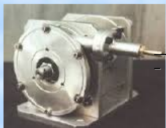
EGG Tesla Turbine 340 kWp Runs on waste heat 177°C to 232°C from exhaust - 650 psig
