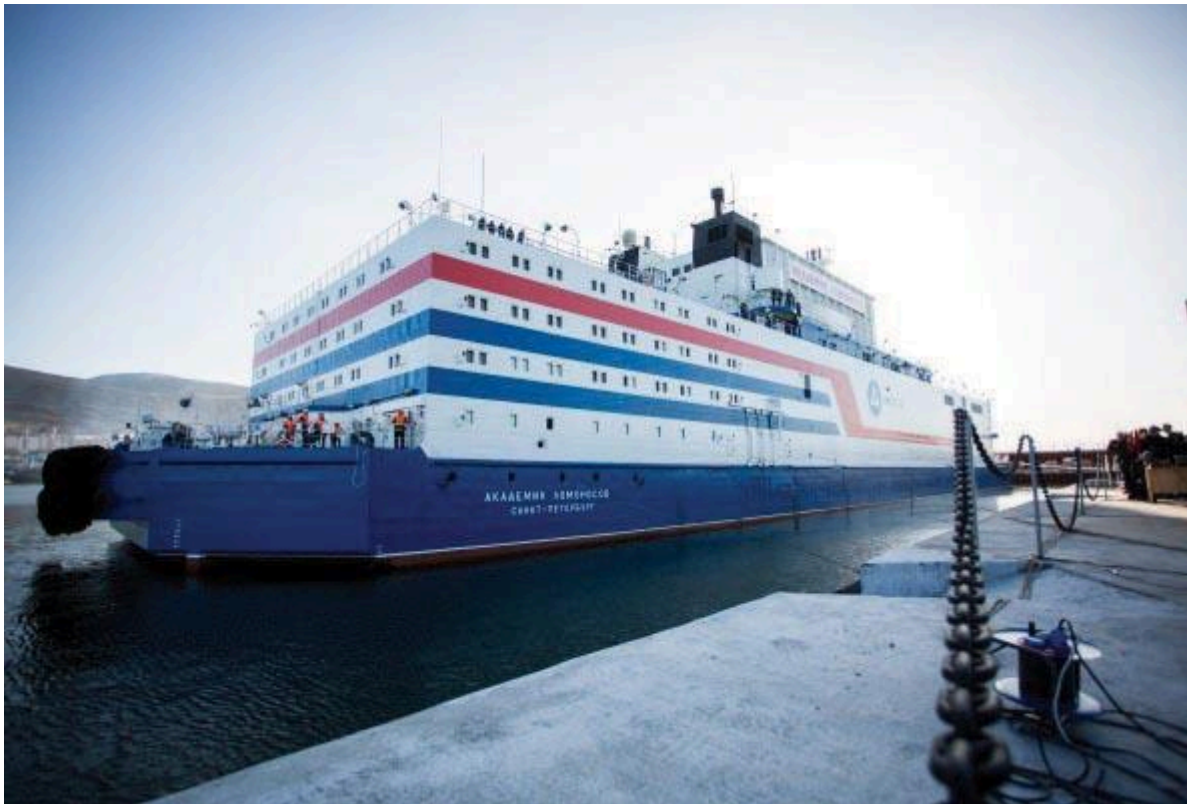
Floating 70 MW Nuclear Power Plant - with 50 Gcal/hr. The plant's length is 120 meters. Ship is 140 x 30 meters.
